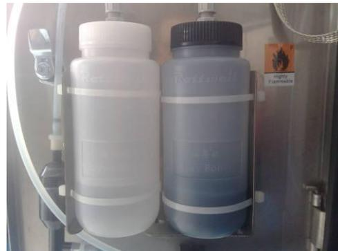
*Fig. 5-3 Solvent bottle & ink bottle in machine*
