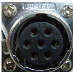
Fig. 6-4 Photo sensor/Alarm output socket
